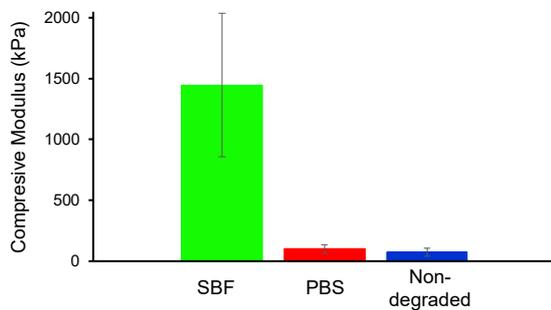
Fig. 9. Compressive moduli of samples with and without degradation.
