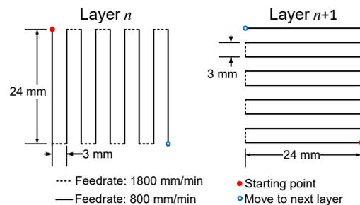
Fig. 2. Printing tool path of the scaffold.
