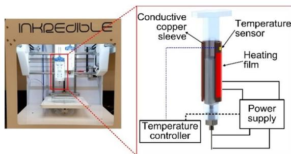
Fig. 1. 3D printing setup with modified printhead
