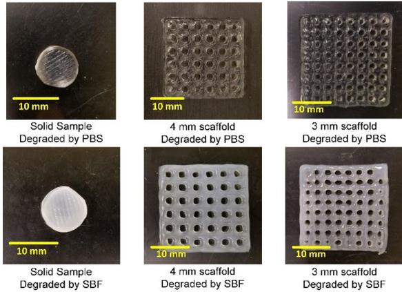
Fig. 5. Samples degraded by PBS (top) and SBF (bottom).
