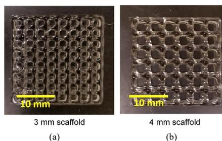
Fig. 4. Fabricated scaffolds: (a) 3 mm scaffold, (b) 4 mm scaffold,
