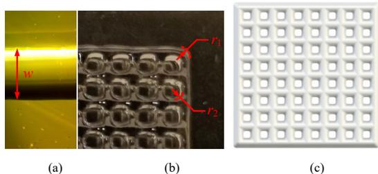
Fig. 3. Reconstruction of the 3D model of the scaffold: (a) line width of the scaffold, (b) corner radii, and (c) the reconstructed 3D model of the scaffold
