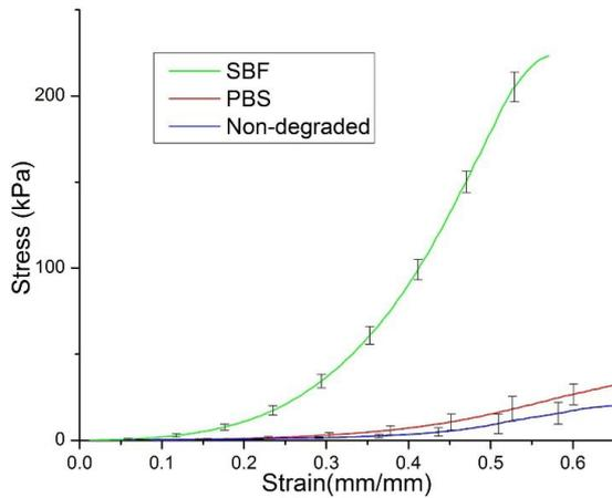
Fig.8. Stress-strain curves of gellan gum samples.
