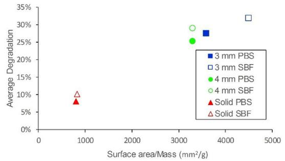
Fig. 7. Ratio of surface area to mass versus average degradation.
